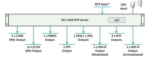
The VCL-2156 is equipped with a highly accurate, low-noise OCXO to provide a high stability, ITU-T G.812, Type II, III compliant holdover clock with better than 12µs accuracy over a 24 hour (5 milliseconds per year) period in the event of unavailability of the GPS / GNSS signal, or GPS / GNSS antenna failure, or a temporary loss of reception in a totally isolated network without any external reference.
